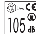
Noise emissions to the surroundings in accordance with the European Union's directive. The machine's emission is stated in the chapter TECHNICAL DATA and on the decals.
